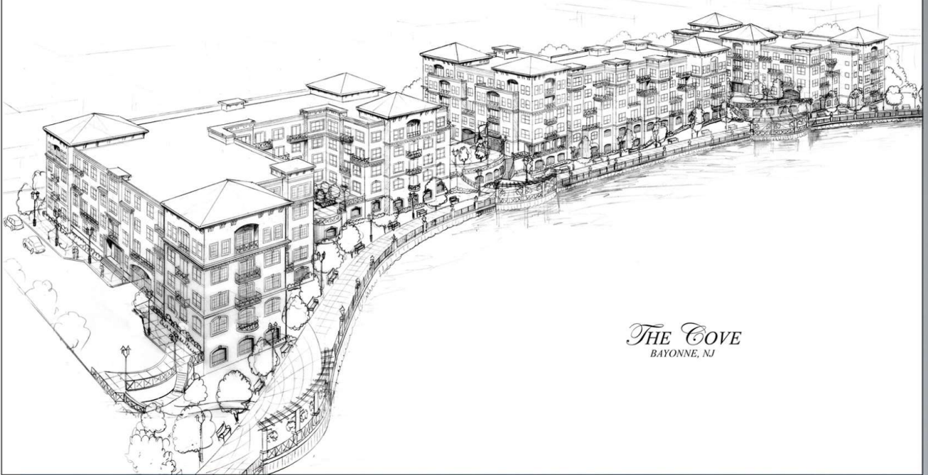
Figure 26-3. A pencil drawing can show a large amount of detail. This is a pencil rendering of a large condominium development. (K.Taylor Architectural Renderings/www.KTaylorRenderings.com; Appel Design Group Architects/www.ADGroupArchitects.com)
